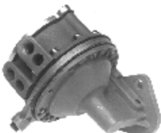
18-7270 AC FUEL PUMP (Flange I.D. #41417, M73019) For: GM (V-8) 305, 350, 400 (5.75 - 7 PSI) Replaces: 21140
