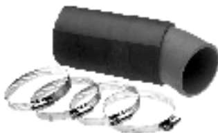
18-1991 30° EXHAUST ELBOW ADAPTER For use with 3" I.D. Exhaust Hose Use 18-1999/AP#5705 Manifold Riser
