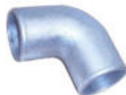
18-1992-1 AP# 5016 80° EXHAUST ELBOW For 3" I.D. Exhaust Hose (As used in 18-1987 Exhaust Manifold Conversion Kit)
