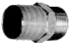
18-4461 AP# 5187 HOSE BARB 3/4" - 14 NPT x 1" Hose Corrosion Resistant Brass Fitting
